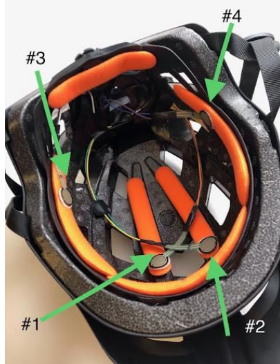
Figure 4: The Cloud Cover on a helmet with the locations of the force sensors shown.
